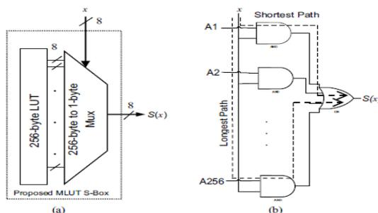
**Fig.6. Multiplexer based S-Box (a) Proposed MLUT S-Box
