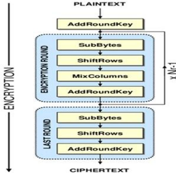
*Fig.1 AES encryption process*
